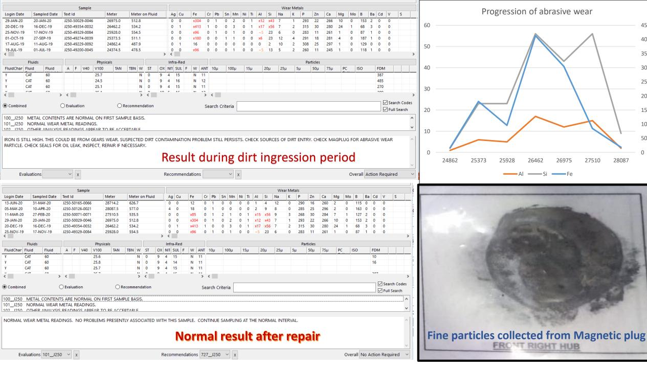
Increase in Aluminium and Silicon are indicating dirt contamination in the system. Fine particles caused by abrasive wear found in magnetic plug. Abrasive wear is the predominant wear mode causing wear in roller race, gears and housing. Machine was inspected and found dirt contamination due to leakage in seals. Components found okay and fit for reuse. Seals and O rings are replaced to resolve this issue. Recheck result found okay.
