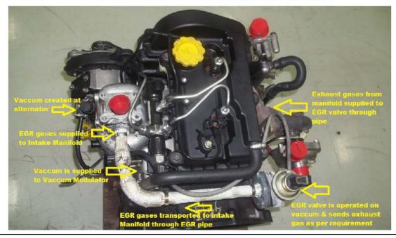
The vaccum operated EGR system doesn't require special maintenance . However the system should be visually inspected for following points at every service interval.
