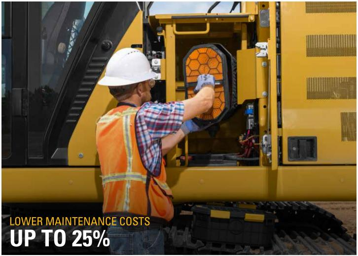
With synchronized and extended maintenance intervals, you get more done at a lower cost compared to the 330D2. Consolidated filter locations make service faster. Hydraulic, air, and fuel tank filters have increased capacity and longer life. Access to the operation and maintenance manual is easy through the in-cab monitor.
