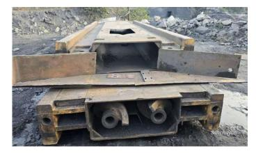
operation on February 17, 2025, during the first shift. This time, the improved modified push beam successfully collected and removed sufficient debris through the auger system to access and free the trapped cutter module. The redesigned system was able to channel fallen material directly into the augers, creating the clearance needed to extract the valuable equipment.
