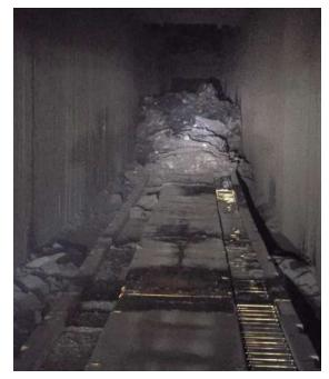
employing two dozers in addition to the machine's own power head to pull out the stuck equipment. This method proved ineffective against the forces holding the cutter module in place. Without a low seam cutter available to assist in the recovery, the team needed to develop an alternative solution to prevent the complete loss of the expensive equipment.
