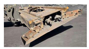
to function as an auger that could collect fallen roof material and transport it out of the hole, thereby clearing a path to the trapped cutter. The design incorporated modifications to standard push beam equipment that would enable it to function as a material removal system.
