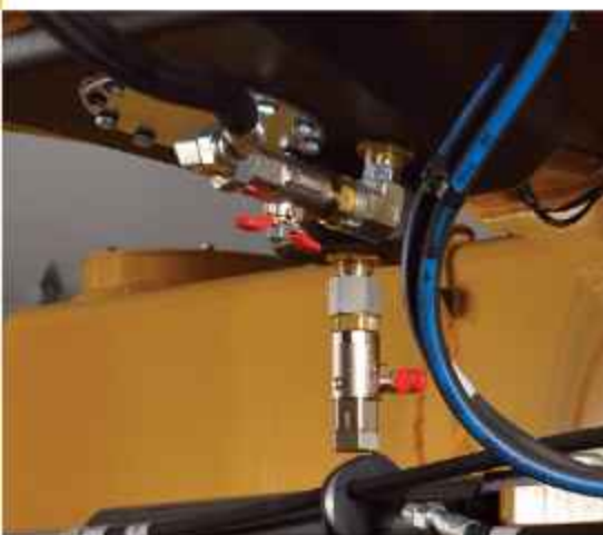
Grouped Drain Valves
