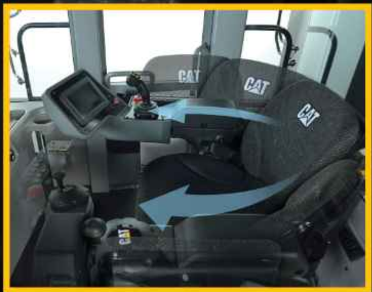
Seat rotates 180 degrees for enhanced comfort and visibility
