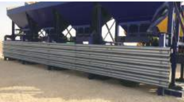
Built-in retaining wall
