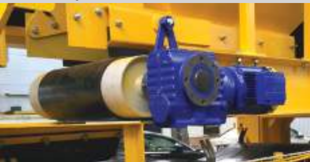
Shaft-mounted inverter-controlled motor
