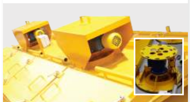
Distributors on Baghouse Filter
