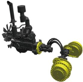
Upgraded hydrostatic system not only leverages Caterpillar automatic, dual path, hydrostatic drive with electronic control technology of the third generation TTT, but also increases efficiency and reliability.
