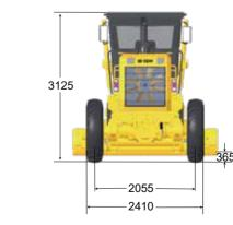
Note: Base (non-ROPS cab,with 13.00-24MP Tube Tire)
